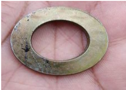
Pic of the washer which was resting in the bottom of the center limb.
