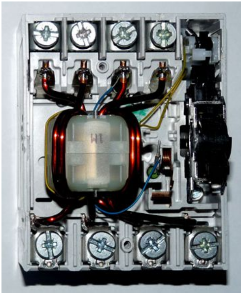
← Internal Construction of RCCB
