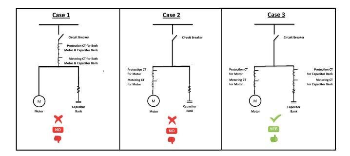
Due to above-described factors, we advise the Plant authorities to modify protection scheme, by implementing separate protection for motors and capacitor bank. We also advise to manipulate the Motor Protection Relay settings by reducing it till the modification in protection scheme is made.
