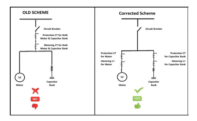
It was common CT and Relays for Both Motors and Capacitor banks which was causing the frequent failure of motors. Here under are the reasons why Common Protection should not be used for HT Motor with Capacitor Banks.
